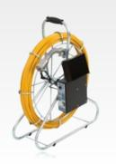
Pipe camera system with Polykat<sup>®</sup> glassfibre profile  $\emptyset$  7.4 mm, length 60 m applicable in pipes from 70 mm up to 500 mm  $\emptyset$  max., suitable with DN 90 up to 100°, stainless steel camera head,  $\emptyset$  50 mm, Nano protected, high marresistant glass, waterproof up to 5 bar max., weight 13 kg
