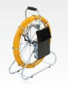
Sewer camera system with Polykat<sup>®</sup> glassfibre profile Ø 9 mm, length 60 m applicable in pipes from 70 mm bis up to 500 mm Ø max., suitable with DN 125 up to 87°, stainless steel camera head, Ø 50 mm, Nano protected, high marresitant glass, waterproof up to 5 bar max., weight 14 kg
