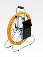
Pipe camera system with Polykat® glassfibre profile  $\emptyset$  7.4 mm, length 60 m applicable in pipes from 50 mm up to 350 mm  $\emptyset$  max., suitable with DN 70 up to 87°, stainless steel camera head,  $\emptyset$  40 mm, high marresistant sapphire glass, waterproof up to 5 bar max., weight 10 kg
